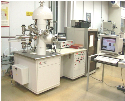
Picture of the AXIS-HS small spot XPS instrument by KRATOS Analytical Ltd. used in the project.
